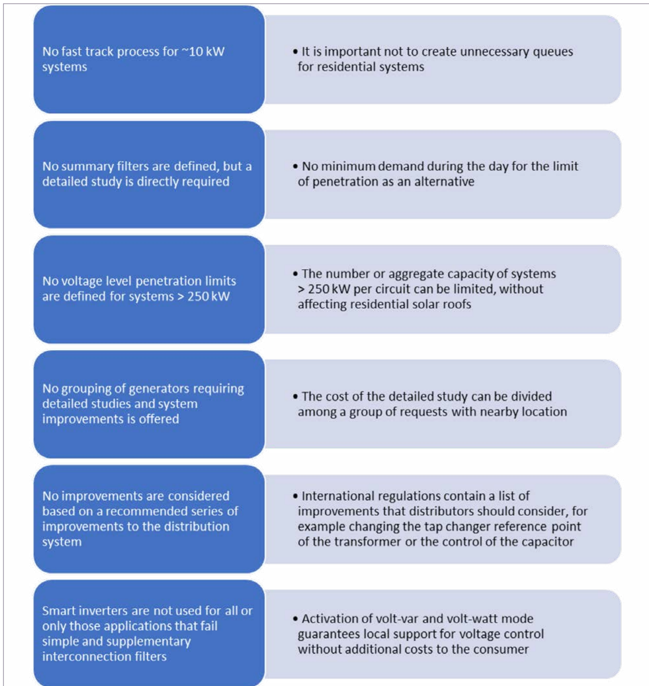
Figure 61: Main differences between the Dominican Republic's interconnection regulations and the best regulatory practices for distributed generation interconnection [15]
